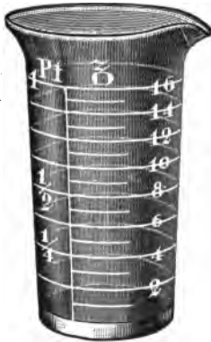
FIG. 1.—Pint Graduate. Graduated on right by ounces, on left by fractions of a pint. The symbol in the center is the symbol for pint.
